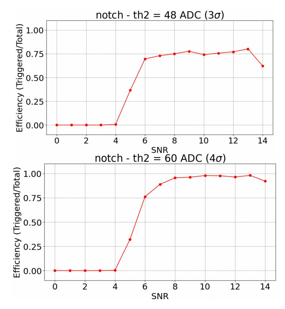
For FIR filter, efficiency decreases significantly at an SNR of 6 and below: need to adjust TH1 parameter
