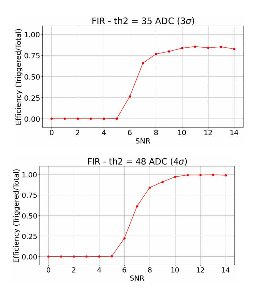
$4\sigma$  is safer than  $3\sigma$ , offering better detection efficiency.
