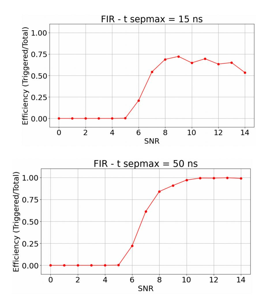
Maximum time separation of 50 ns provides better efficiency than 15 ns.
