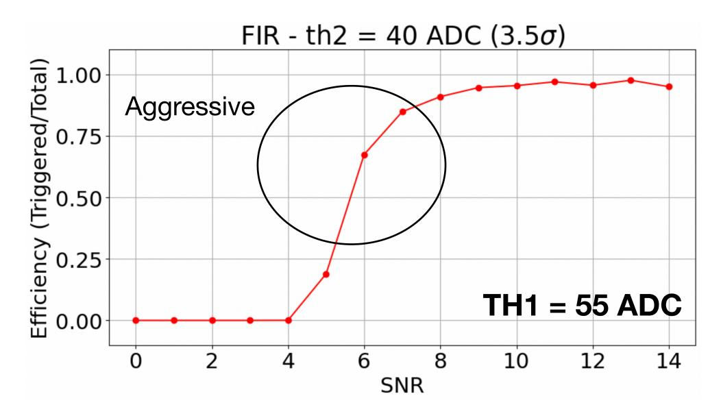
**Optimal parameters**  $t_quiet = 500 \text{ ns}, t_period : 500 \text{ ns}$  $NC = [2-7], t_sepmax = 50 ns$ • For FIR: **TH1 = 55 ADC** and TH2 = 40 ADC (3.5 $\sigma$ ) or 48 ADC (4 $\sigma$ ) • For notch: **TH1 = 70 ADC** and TH2 = 60 ADC (4 $\sigma$ )
