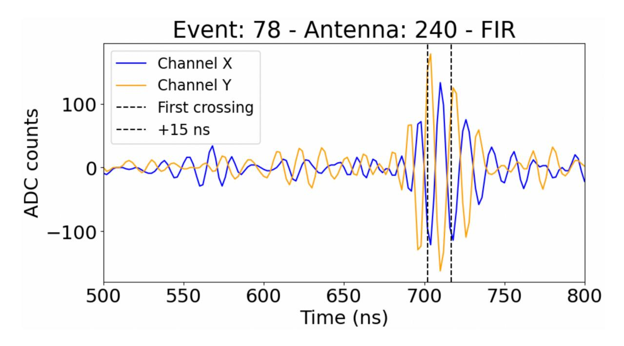
With t\_sepmax = 15 ns, time window still overlaps with first pulse in some cases — too short to reach a second pulse
